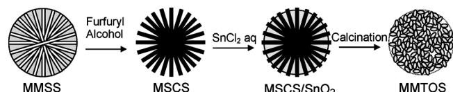
Scheme 1. Nanocasting Route To Obtain MMTOS a
